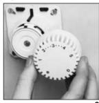
Turn the centre adjustment screw clockwise until stop, then turn it anticlockwise until the factory red paint mark falls in line with the 'stop rib'. Then replace the graduated scale cap so that the number (4) also falls in line with the 'stop rib'. Thus the original setting is restored.
